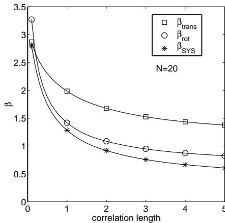
Figure 10. Component and system reliability indices for the pile group with lognormal cohesion field.
