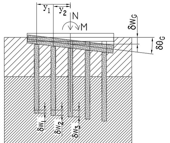
Figure 1. Pile group: virtual displacement field.
